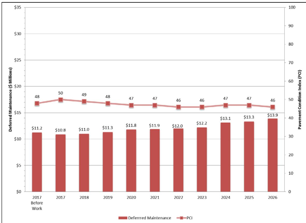
**Figure 6: PCI vs Deferred Maintenance for Scenario 1**
