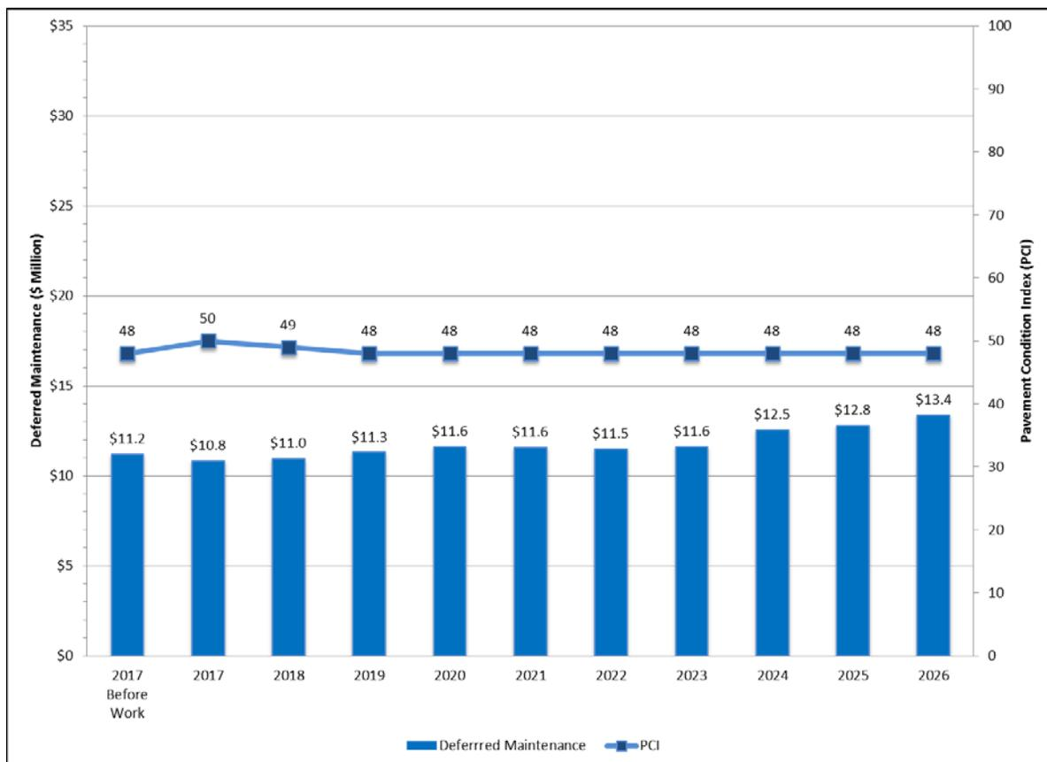
Figure 7: PCI vs Deferred Maintenance for Scenario 2
