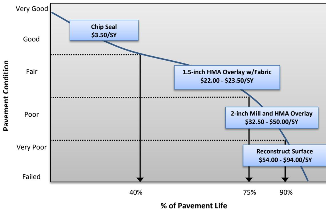
Figure 5: Costs of Maintaining Pavements over Time
