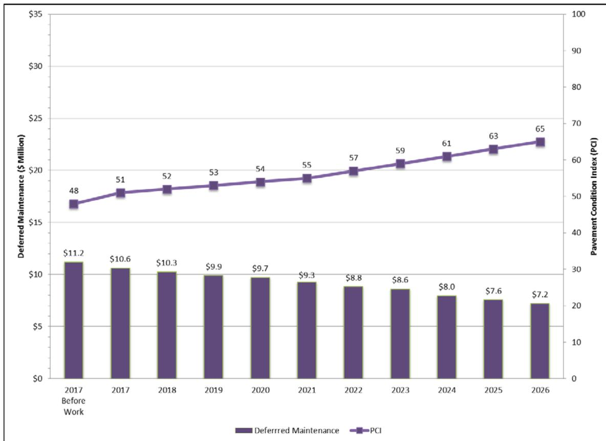
Figure 9: PCI vs Deferred Maintenance for Scenario 4
