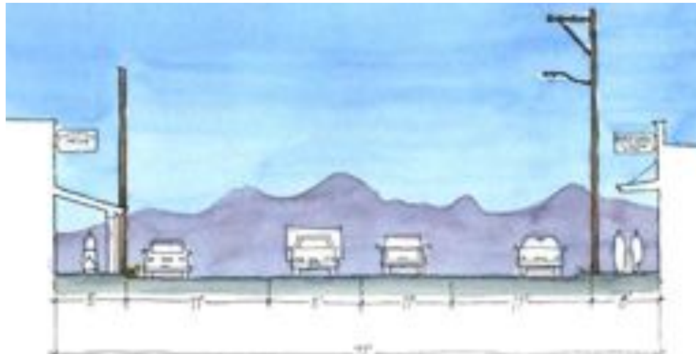
Existing right-of-way shows two 11' travel lanes, wide shoulders with informal, on-street parking. Sidewalks are in various states of disrepair.
