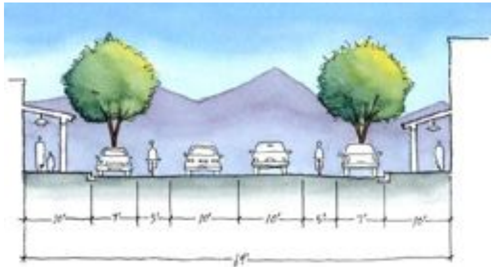
Improved 64' ROW illustrates two 10' travel lanes, 5' bike lanes, 7' parallel parking lanes, and 10' improved sidewalks.
