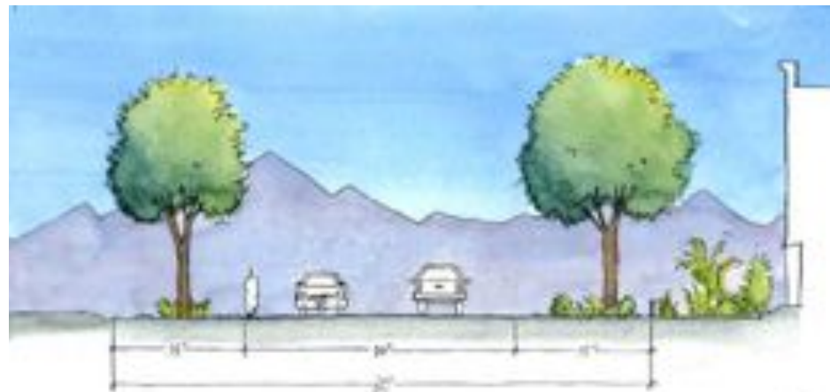
Existing right-of-way shows two 15' travel lanes, narrow shoulders of gravel/dirt and no sidewalks.
